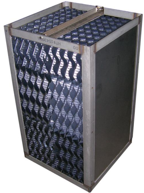
Hydro Quip's UNIPACK coalescing media is a cross-fluted type media, consisting of parallel corrugated plates. It is specially designed to provide highly efficient liquid/liquid and liquid/solid separation due to its high surface area to volume ratio.
